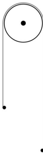
Figure 37 Rotatable wheel dividing the string in two segments
