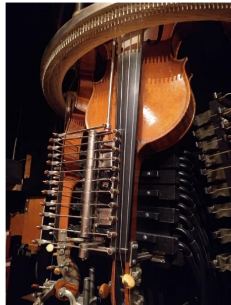
Figure 5 The circular rotating bow mechanism used in the Hupfeld Phonoliszt Violina is similar to bowing mechanism in Hurdy Gurdy. It consists of a disc that rotates infinitely and excites the string with friction.
