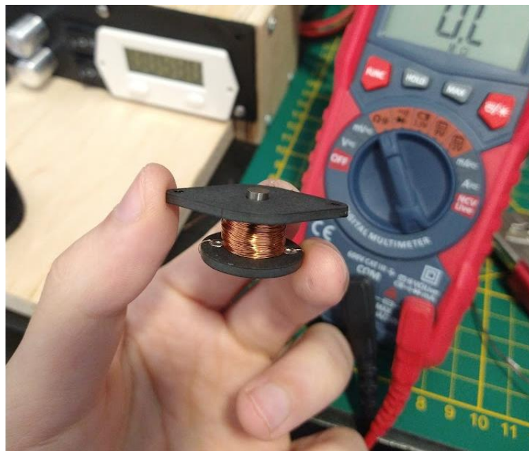
Figure 39 Hand-made 8 ohm coil with fibre frame and Alnico magnet core
