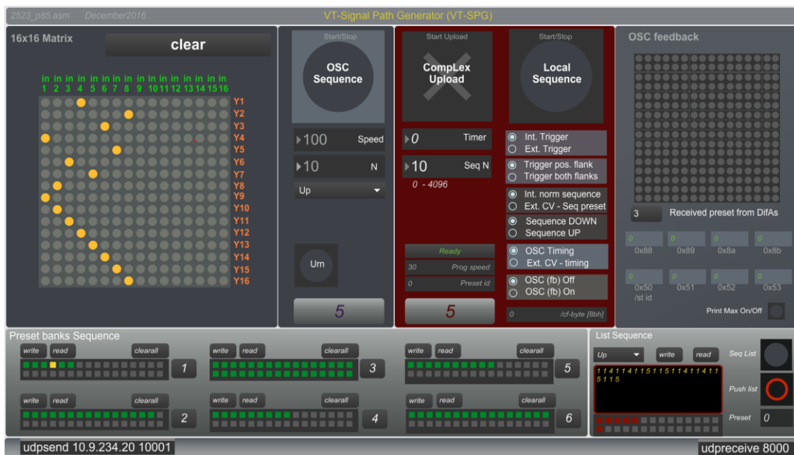
Figure 45 MAX MSP patch to control the Signal Patch Generator. User can make connections between the 16 Inputs and 16 Outputs by selecting dots in the matrix array.
