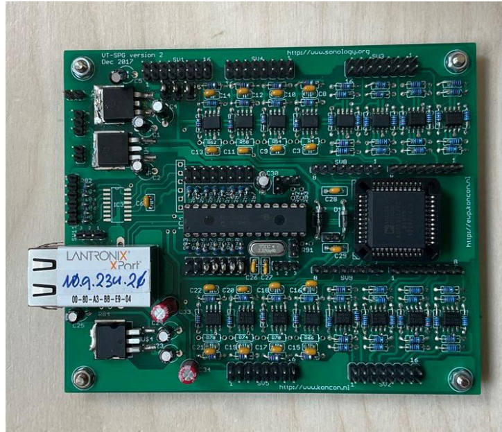
Figure 44 Signal Path Generator PCB designed by Lex van den Broek
