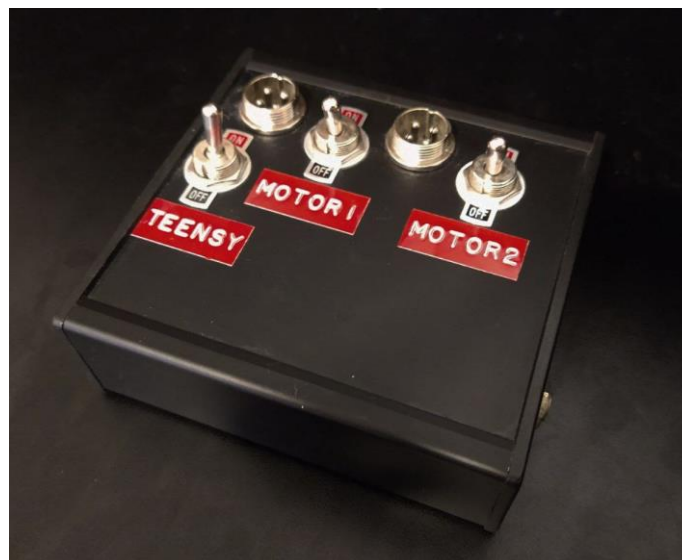
Figure 24 stepper motor driver breakout box
