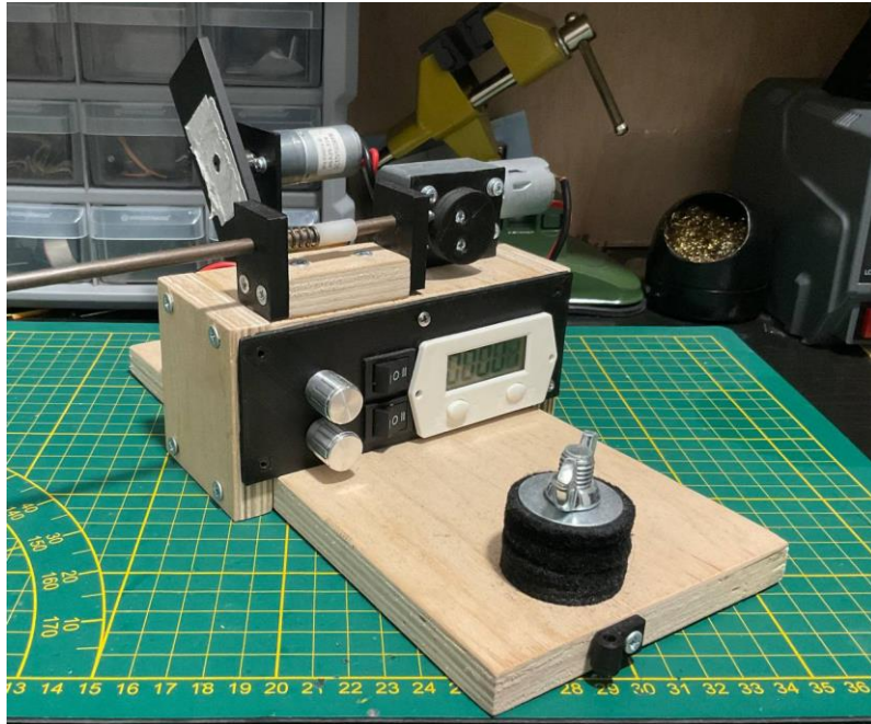
Figure 38 Hand-made pickup winder
