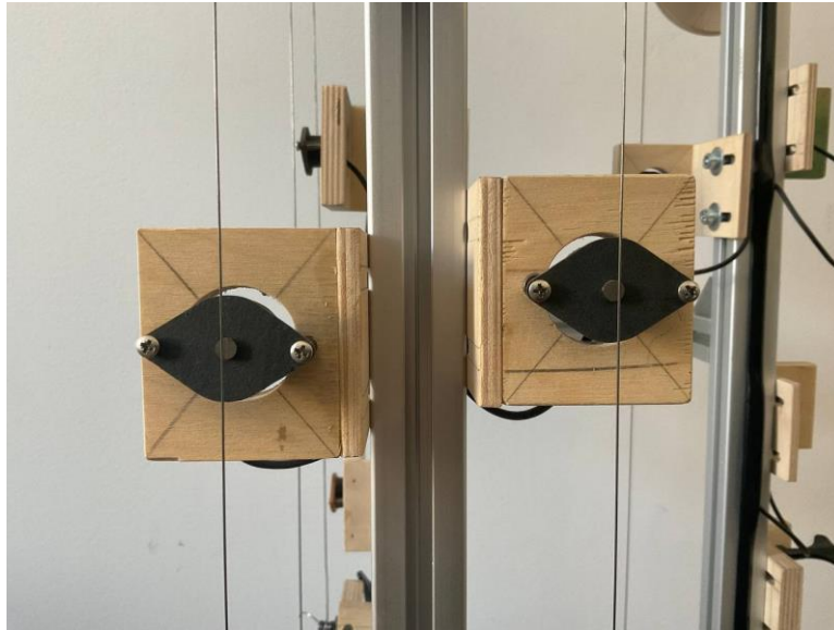
Figure 40 Output coils installed on the modular frame
